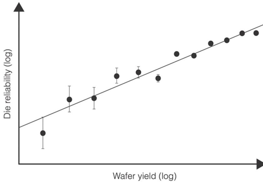
Figure 1. Data demonstrating the strong correlation between IC device reliability and yield.<sup>1</sup>
