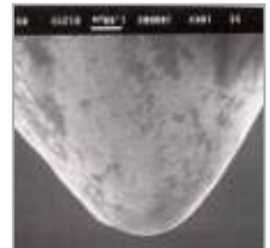
Figure 4. The standard KLA stylus has a 2 \mu m radius with a 60° included angle.
