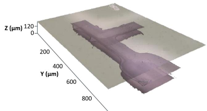
**Figure 5.** Zeta image of a closed microfluidics channel with a transparent cover plate, showing the top, middle, and bottom surfaces. The cover plate thickness measured 93.4µm, and the channel depth measured 59.2µm.
