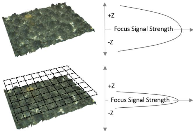
**Figure 2.** Without ZDot technology (top), the focus signal strength has a wider peak, making it difficult to detect the exact focus height. With ZDot technology (bottom), the exact focus height is determined as the center between the two Z heights of maximum contrast. Note that in optical terms, the signal peak of the Zeta system is narrower than that of a regular optical microscope, but enhanced focal detection is possible because of the 1000s of signal points from the ZDot array.
