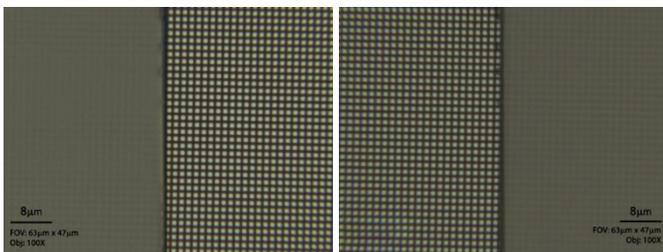
**Figure 3.** ZDot technology maximizes signal strength at multiple focal planes in order to provide accurate step height measurements. The left image shows the ZDot grid in focus at the top surface of the step (right side of image), and the right image shows the grid in focus at the bottom surface of the step (left side of image).
