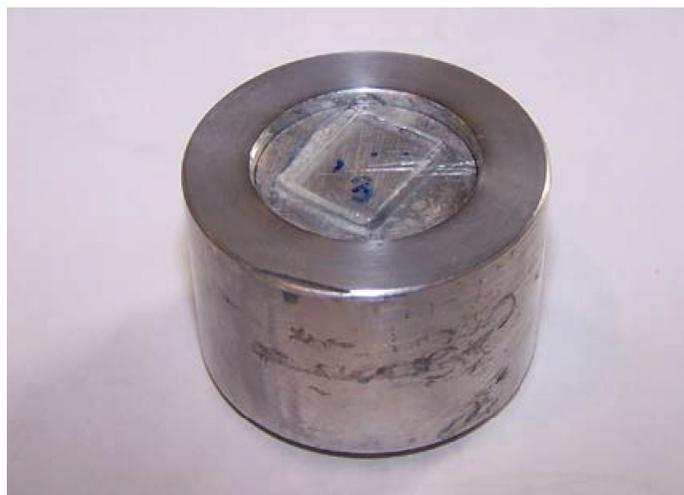
Figure 1. Fixed mouse lung cells mounted in a fluid puck for scanning and testing with the Nano Indenter G200 system.
