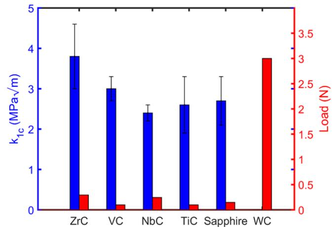
Figure 2. (top) SEM images of residual impressions for six hard materials: NbC, sapphire, VC, TiC, ZrC, and WC; (bottom) calculated fracture toughness  $K_c$  and maximum applied load for the six materials.
