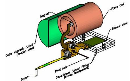
**Figure 4** P-Series Sensor Schematic
