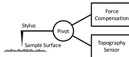
**Figure 1** Stylus Profiler Sensor Schematic
