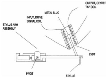
**Figure 2** ASIQ Sensor Schematic
