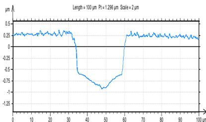
**Figure 4:** Isolation Scribe measurement in the Mo electrode.
