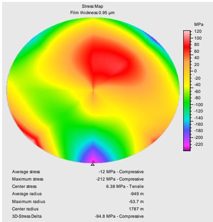
**Figure 5:** Typical 3D stress measurement after film deposition.
