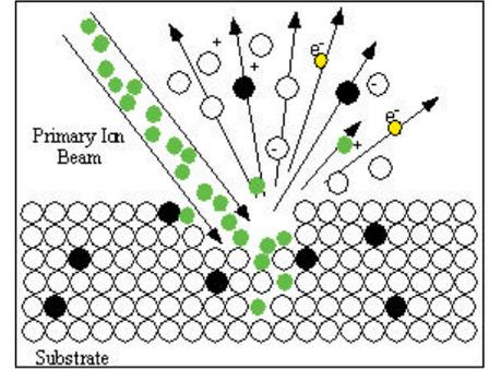
Fig. 2. Bombardment of a sample surface with energetic primary ions. The sputtered impurity and substrate ions are represented by black and white colors respectively.
