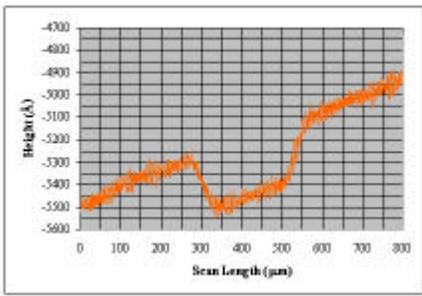
**Fig. 4.** An unlevelled trace, indicating that the substrate is not flatly seated on the profiler stage.
