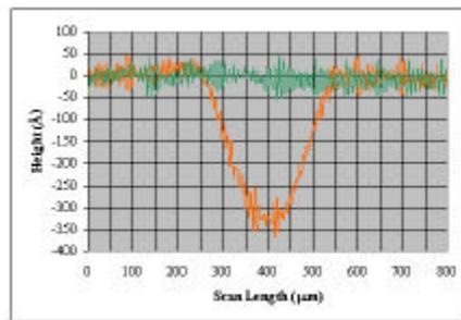
Fig. 3. Comparison of noise to a SIMS crater depth measurement.
