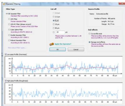
Figure 8 2D Roughness/Waviness Operator
