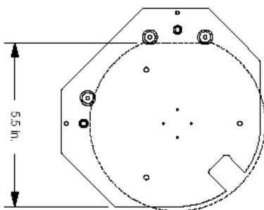
**Figure X.** 6-inch (150mm) flat or square substrate locator for Stress measurements.
