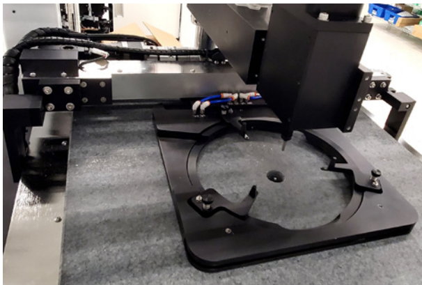
Non-contact, dual sensor wafer measurements are acquired on non-contact, air bearing stage
