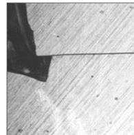
Silicon  $\mu$ Crack
