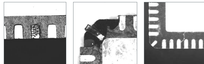
Bleed on Pad Chipped Edge Package Cracks or Scratches
